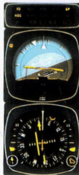
**4.** The heading "bug" has been previously set to the missed approach heading, 90°. Activating the HDG mode will cause the Command V-bar in the FCI to command a turn to that heading. Pitch-up attitude may be adjusted from the Go-Around angle by using CWS or the Vertical Trim control on the Autopilot controller, either of which terminates "GA" mode.
