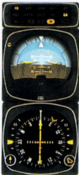
**3.** At the Middle Marker a missed approach is executed by pressing the Go-Around button on the throttle as you increase power. This disengages the Autopilot and the FCI commands the correct nose-up attitude and wings level. At the discretion of the pilot, the Autopilot may be reengaged to complete the missed approach. (Some airplanes are certified with autopilot remaining engaged when GA selected.)
