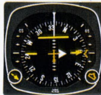
4. Halfway through your turn to the inbound 064° course, the KI 525A shows the symbolic aircraft approaching the deviation bar at a right angle. By keeping the top of the deviation bar on the lubber line, you can complete your turn and roll out precisely on course.
