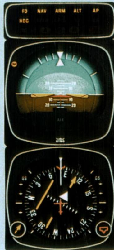
2. A waypoint has been established and the RNAV computer is in ENROUTE mode. A 112° course to the waypoint has been selected and NAV mode pushed "on". HDG and NAV/ARM modes are activated for automatic capture of the 112° course to the waypoint. The capture rate is now being computed based on closure rate. The airplane must be headed toward the selected course in order for NAV/CPLD to occur.
