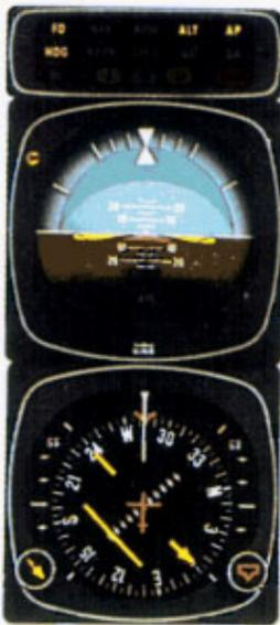
3. During the procedure turn outbound the deviation bar shows pictorially that the aircraft is flying away from the Localizer centerline at a 45° angle on a selected heading of 283°.
