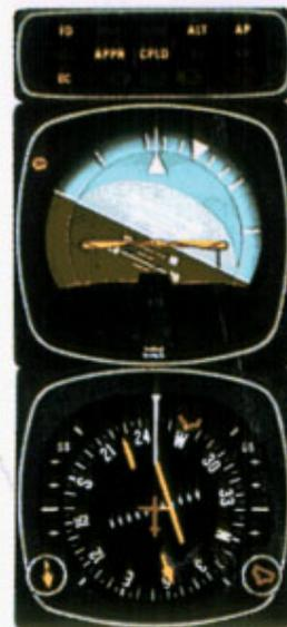
2. When the computed capture point is reached the APPR CPLD mode is automatically activated and a left turn outbound on the localizer is commanded by the FCI, and is satisfied by the Autopilot.
