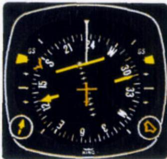
1. You are vectored from the holding pattern to the 13-mile DME arc. The aircraft is turning, with the heading bug set on 170° to intercept the Localizer. You have already set the selected course pointer on the inbound ILS course 130° and the KI 525A shows the Localizer course is directly ahead. The Glide-slope pointers came into view when the ILS frequency was tuned, since a usable Glide-slope signal is being received.
