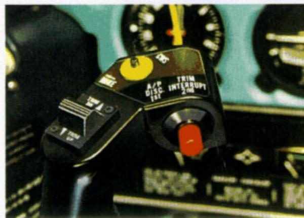
while Autopilot control functions and Pitch Command and Altitude Hold modes are synchronized so that, upon release of the CWS mode button, the Autopilot will smoothly reassume control of the aircraft to the original lateral command and existing vertical command.
