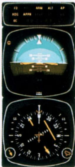
1. In HDG SEL and ALT Hold mode on a LOC channel, the aircraft is heading 270° toward the Localizer. The front inbound localizer course of 58° is selected. APPR mode and "BC" have been selected. The back course (BC) mode is selected to go outbound on the front course. The capture point is now being computed, based on closure rate.
