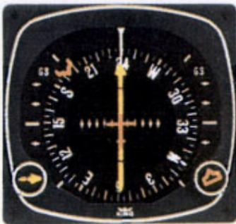
1. You are outbound on the back Localizer course, having already set the course pointer to the inbound front course at 238°. The heading bug is preset at 193° for the procedure turn. (Since there is usually no Glideslope signal on a back course, the Glideslope pointers are out of sight.)
