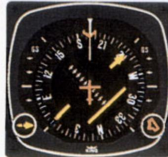
2. During the procedure turn outbound, the deviation bar shows pictorially that the aircraft (as represented by the symbolic aircraft in the center of the KI 525A) is flying away from the Localizer centerline at a 45° angle when the heading marker is under the lubber line. Note that left-right deviations of the course bar give "fly-to" indicators, just as on the front course.
