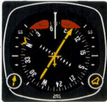
The KI 525A Pictorial Navigation Indicator is the panel display for the KCS 55A Compass System. It combines the functions of the standard directional gyro and the VOR/LOC/Glideslope deviation indicator.
