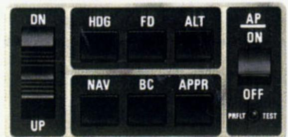
The KC 291 Yaw Mode Controller is installed adjacent and to the right of the KC 290 Mode Controller when the optional yaw (rudder) axis is included in the KFC 200 system. The yaw axis is wired so that it automatically engages when the Autopilot is engaged. Disengagement of the yaw damper is accomplished by pushing the button on the KC 291 or the A/P disconnect on the control wheel.
