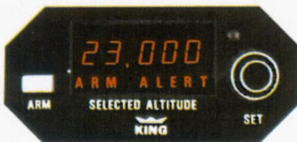
As the aircraft approaches the selected altitude, an "adaptive" pitch rate command will automatically guide the pilot through it at a low rate. As the aircraft reaches the selected altitude, ALT HOLD will automatically engage, "ALT" will light on the Annunciator Panel and "ARM" will disappear on the KAS 297. The command bars on the FCI will call for level flight at the selected altitude. If autopilot is engaged, the system will perform the required maneuvers.
