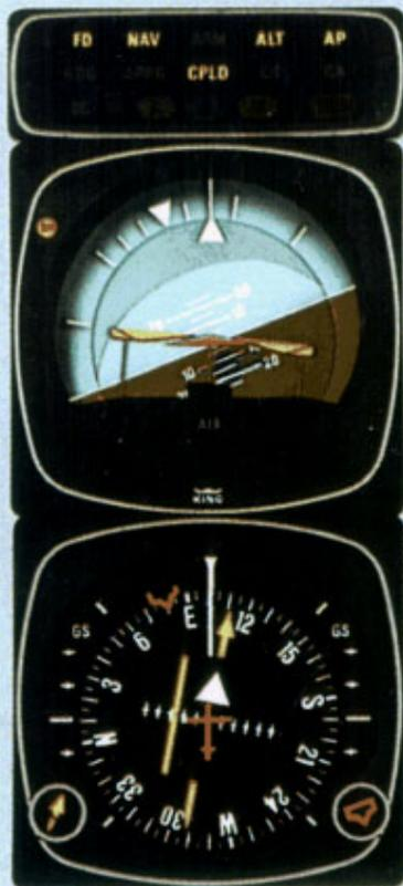
3. Capture sequence starts when NAV/CPLD mode is automatically engaged, cancelling the NAV/ARM and HDG modes. The Command V-bar will call for a right bank which is being satisfied by the Autopilot.
