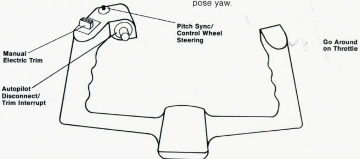
**Typical Control Wheel Switch Arrangements**
