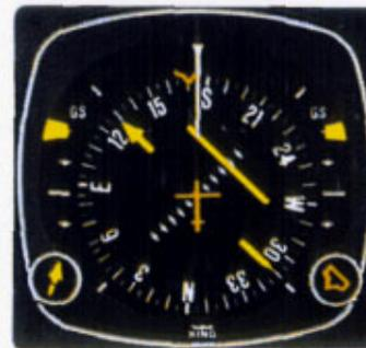
2. Capturing the ILS course can be accomplished without overshooting or bracketing with the same technique you used in intercepting an enroute course: Simply keep the top of the deviation bar on the lubber line and coordinate your turn until the bar is centered with the course arrow. Each dot on the LOC deviation scale represents 1/2° deviation when tuned to an ILS frequency.
