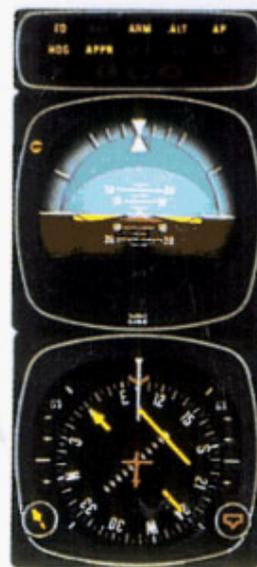
4. Now you have reset the heading select bug to 103° and made a 180° turn to this heading. This 103° heading will intercept the front course. You must now reselect Approach mode by depressing the APPR button on the Mode Controller. The PNI clearly pictures the course you are to intercept and the angle of interception. APPR ARM mode has been selected so that automatic capture of the Localizer will occur.
