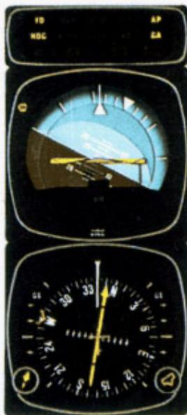
**3.** With the Autopilot engaged, the aircraft is responding to the FCI commands with a left bank. Takeoff climb attitude continues. (Desired altitude may now be selected and armed on the optional KAS 297 altitude selector. Altitude alerting will be provided as you approach your selected altitude.)
