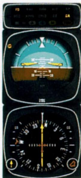
1. The FD has been engaged. Takeoff is in the GO-AROUND mode, activated by depressing the GO-AROUND button located on the throttle. "GO-AROUND" is lighted on the annunciator panel. Wings are commanded level and the nose up to the GO-AROUND angle. Takeoff is on runway 35 as shown on the PNI.
