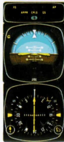
2. The Autopilot (or pilot) is following the Command V-bar on the FCI which command the necessary heading to maintain on center-line of the Localizer. At the Outer Marker the Glideslope pointers are approximately at midpoint. Altitude Hold is automatically disengaged and Glideslope capture occurs when the airplane passes thru beam center. The V-bar will command a descent on the Glideslope and on Localizer.
