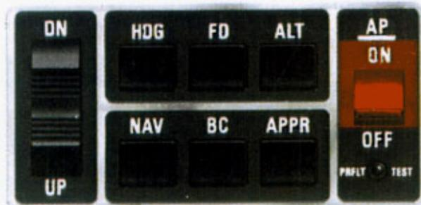
**CAUTION:** Overpowering the Autopilot in the pitch axis in flight for periods of 3 seconds or more will result in the autotrim system operating in the direction to oppose the pilot and will, therefore, cause an increase in the pitch overpower forces, and if Autopilot is disengaged, will result in a pitch transient control force. Operation of the Autopilot on the ground may cause the autotrim to run because of backforce generated by elevator downsprings or pilot induced forces.
