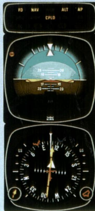
4. The aircraft has completed its turn to the 112° course. A wind correction produces an aircraft heading of 105°, displaying a 7° "crab" angle to maintain the 112° course.
