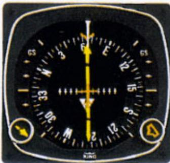
1. Approaching the STL VORTAC, the controller asks you to hold southwest of the VORTAC on the 244° radial, right turns. You are now over the station with a 064° course selected (the TO/FROM indicator has swung to "FROM"). Set your heading bug to the reciprocal or outbound heading of 244° for easy reference and begin your right turn holding pattern.
