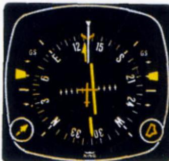
3. The KI 525A shows you that you have intercepted the Localizer course. The Glide-slope pointers have started to center, although the display indicates your aircraft is still below the glidepath at this point.
