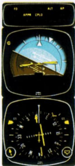
1. Continuing the maneuver on preceding page, APPR coupling occurs and the Glideslope mode is automatically armed. The Command V-bar will command a turn to the LOC course and the PNI shows your position in relation to the LOC course.
