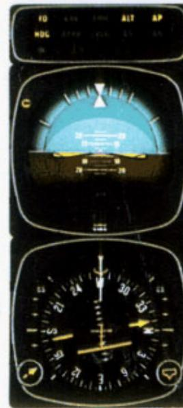
**4.** Desired altitude has been reached, ALT HOLD mode has been engaged and the aircraft has returned to level flight. The 270° heading has been acquired.
